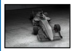
As the next step up from F4 competition, the all-new F3 Americas car will demand more of drivers, and features more configurable aero components, 2018-spec impact safety structures, increased engine power, and more sophisticated data acquisition.
